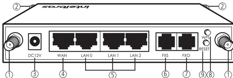
1. Conectores para as antenas GSM/LTE.
