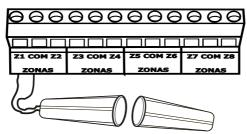
5. After installation, check if, by moving the magnet away from the reed switch, the alarm panel goes off, indicating that there was a tampering. If necessary, adjust the position of the sensor.
