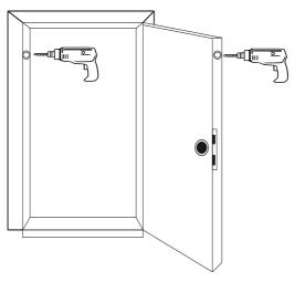
2. Attach the magnet to the moving part and the reed switch to the attached part of the structure.
