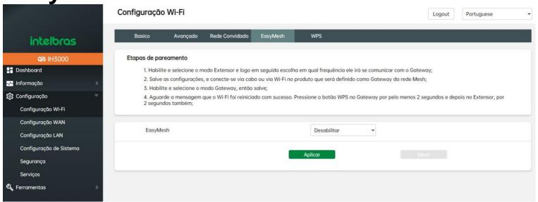
On this screen, you configure EasyMesh, where you can create a mesh network using the GX 3000\* and IH 3000.
