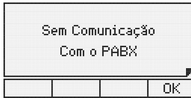
Terminal without communication with the PABX
