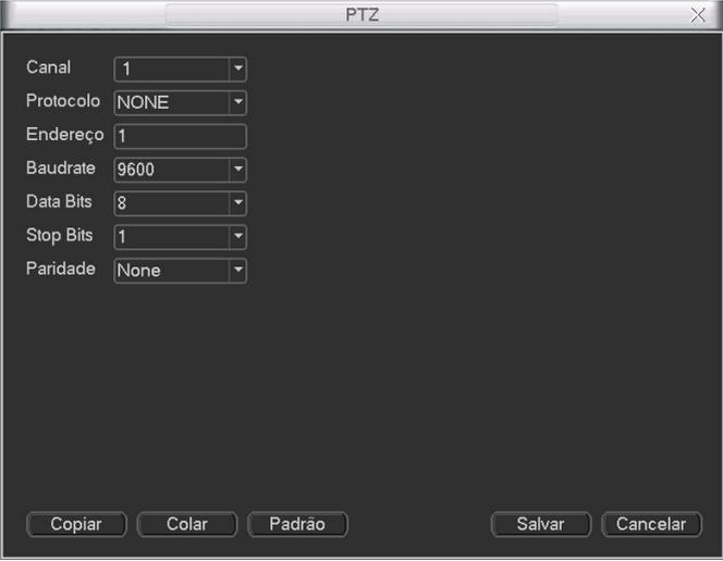
The image shows a software window titled "PTZ" with a close button (X) in the top right corner. The window contains a configuration interface with the following elements:
