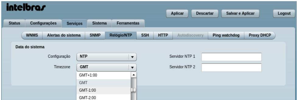
The screenshot shows the Intelbras web interface for NTP configuration. The 'Configuração' dropdown is set to 'NTP'. The 'Timezone' dropdown is open, showing options: GMT+1:00, GMT, GMT-1:00, and GMT-2:00. There are two input fields for 'Servidor NTP 1' and 'Servidor NTP 2'.
