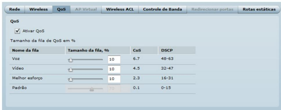
The screenshot shows the QoS configuration page with the 'Ativar QoS' checkbox checked. Below it, a table lists the queue configurations:
