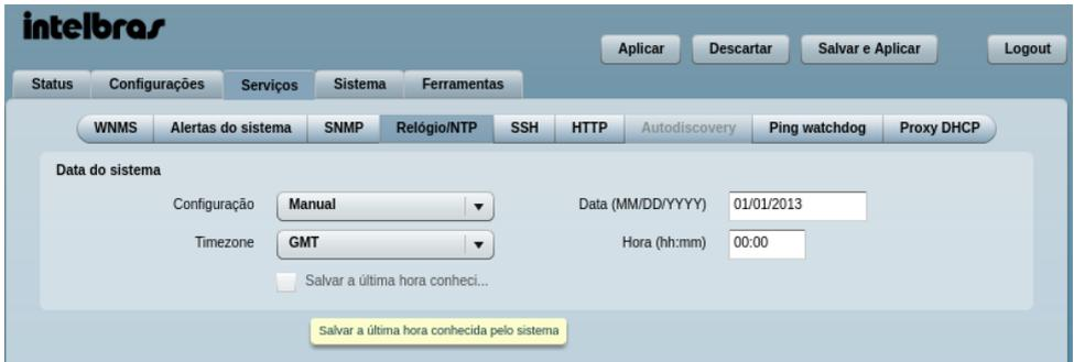
The screenshot shows the Intelbras web interface for NTP configuration. The 'Configuração' dropdown is set to 'Manual'. The 'Data' field is '01/01/2013' and the 'Hora' field is '00:00'. The 'Timezone' dropdown is set to 'GMT'. There is a checkbox for 'Salvar a última hora conhecida...' and a button 'Salvar a última hora conhecida pelo sistema'.
