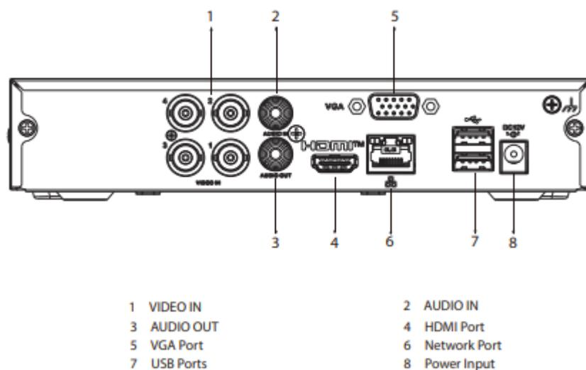
Figura 1 - Painel MHDX 1204-C Dual audio
